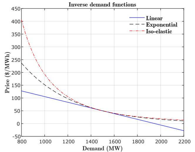
Fig. 8: Calibrated linear, exponential and iso-elastic inverse demand functions at price 50 \$/MWh, demand 1500 MW, and elasticity -0.3.
