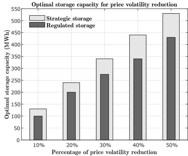
Fig. 3: Optimal strategic and regulated storage capacity for achieving different price volatility levels in SA region for a high demand day with coal-plant outage.
