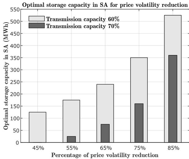
Fig. 6: Optimal regulated storage capacity versus the percentage of price volatility reduction in the two-node market in a high demand day with coal-plant outage in SA.
