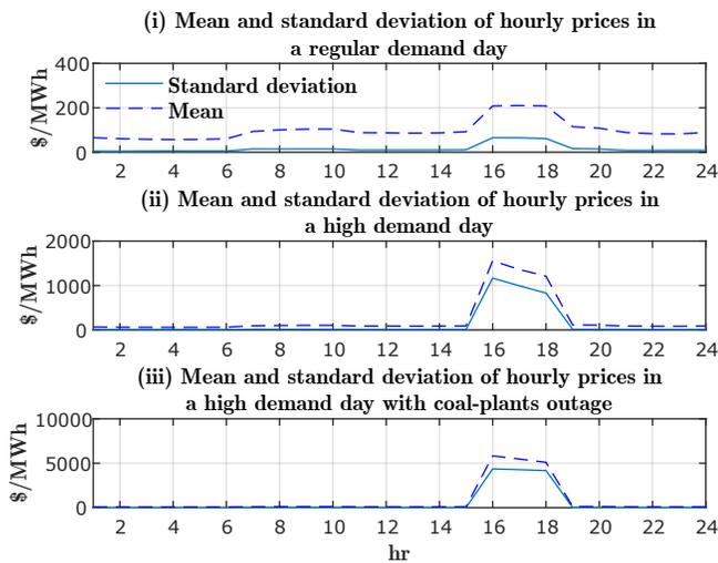
Fig. 2: Standard deviation and mean of hourly wholesale electricity prices in SA with no storage.
