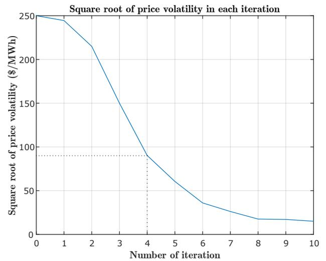
Fig. 7: Square root of price volatility level in the 30-bus system after ten iterations of Algorithm 1 with  $\Delta Q^s = 15\text{MWh}$ .
