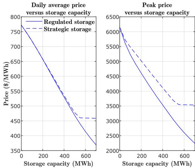
Fig. 4: Daily peak and average prices in SA versus storage capacity in a high demand day with coal-plant outage.
