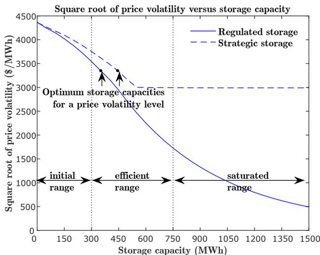
Fig. 5: Square root of price volatility in SA versus storage capacity during a high demand day with coal-plant outage.
