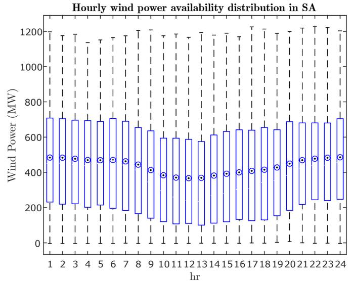
Fig. 1: SA’s Hourly wind power availability distribution in 2015 (the central marks show the average levels and the bottom and top edges of the boxes indicate the 25th and 75th percentiles).
