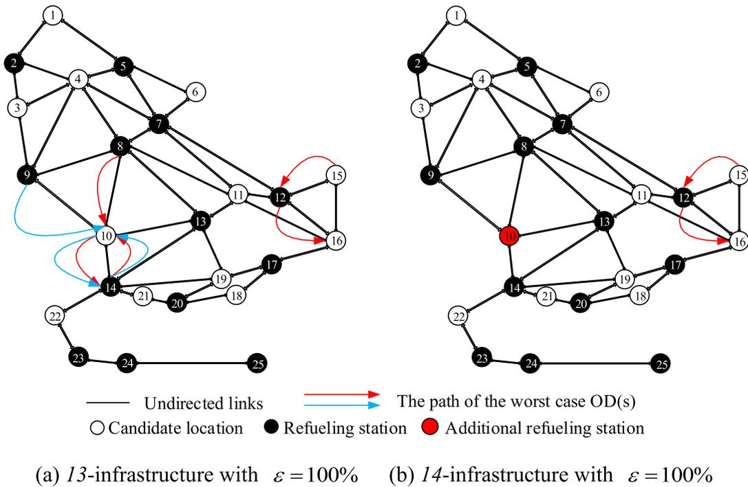
Fig. 8. Sensitivity analysis of the number of refueling facilities for a vehicle range of 10.
