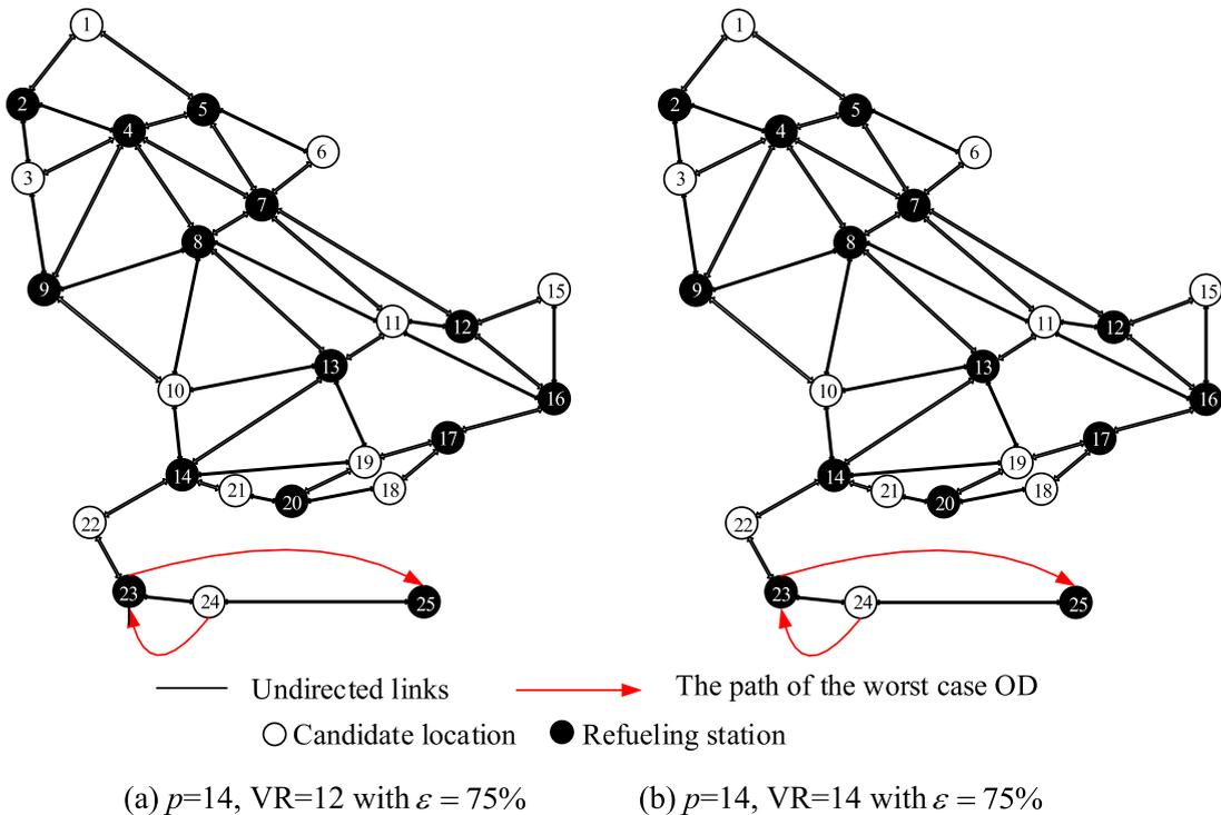
Fig. 10. The optimal infrastructure for vehicle ranges of 12 and 14 for  $p = 14$ .
