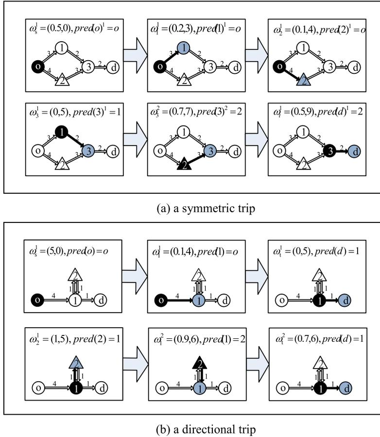
Fig. 1. Two illustrative examples of the VRCS algorithm.
