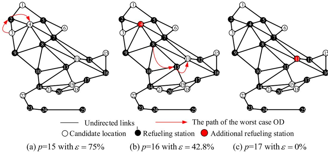
Fig. 9. The optimal infrastructure for  $p = 15, 16, 17$  for a vehicle range of 10.
