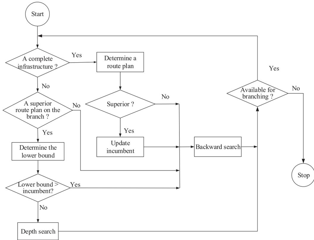
Fig. 4. Flowchart of the implicit enumeration algorithm.
