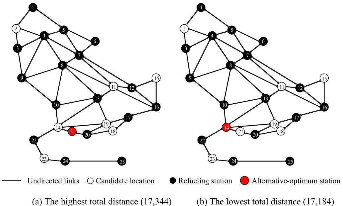
**Fig. 6.** An illustration of multiple optimal solutions for 18-infrastructure.
