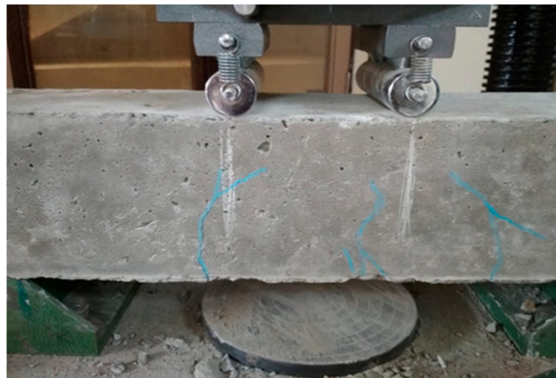
Figure 6. Loading setup on beam.
