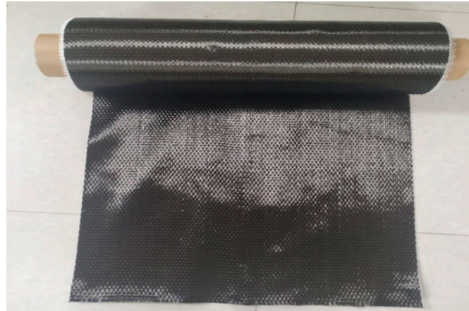
Figure 5. CFRP sheets (Sika wrap-230C).
