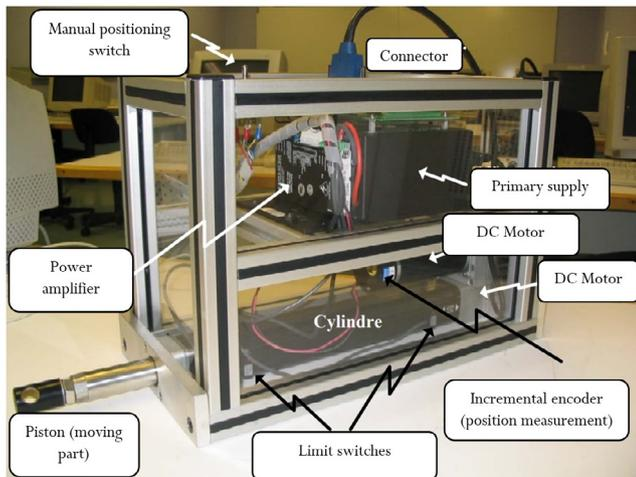
Fig. 6. Electric Cylinder.
