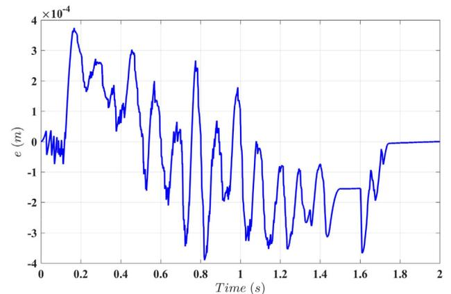
Fig. 12. Tracking error of proposed PRL performance (related with Fig. 11).
