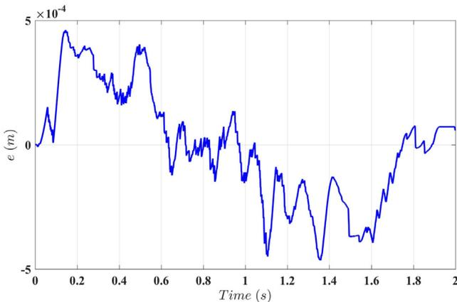
Fig. 9. Tracking error of SMCERL performance (related with Fig. 8).
