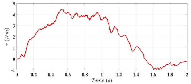
Fig. 10. Control input of SMCERL performance (related with Fig. 8).
