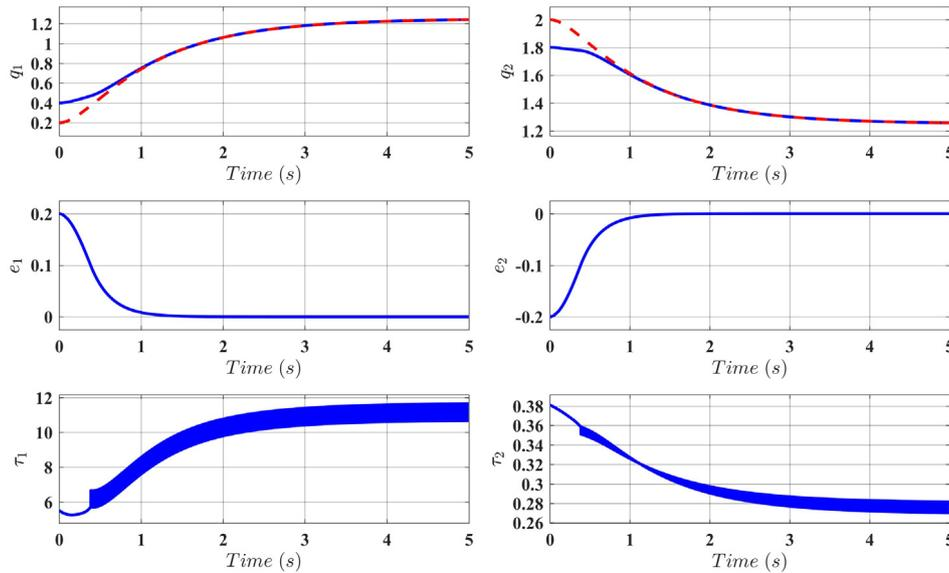
Fig. 3. Evolution tracking of Sliding Mode Controller with Exponential Reaching law (SMCERL).
