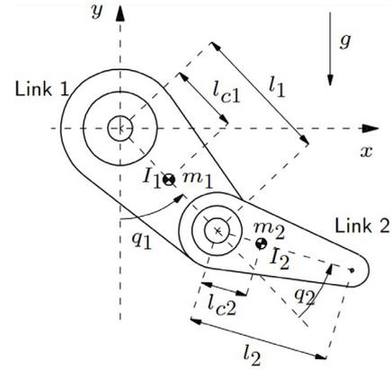
Fig. 1. Two-link of the Pelican prototype robot [23].
