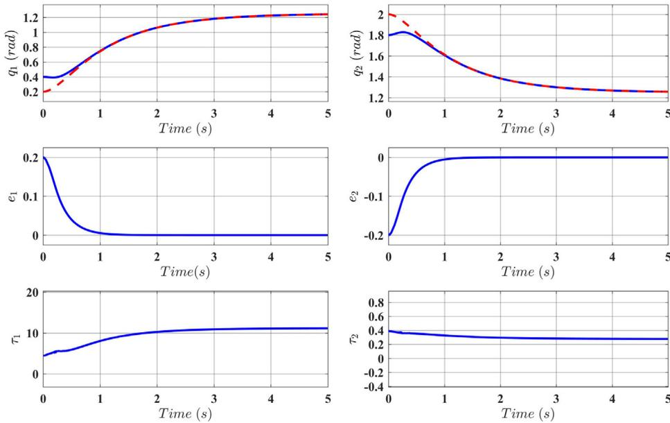
Fig. 4. Evolution tracking of Sliding Mode Controller with proposed reaching law (PRL).
