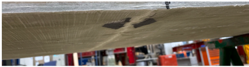
Fig. 8. Failure mechanism due to fatigue.
