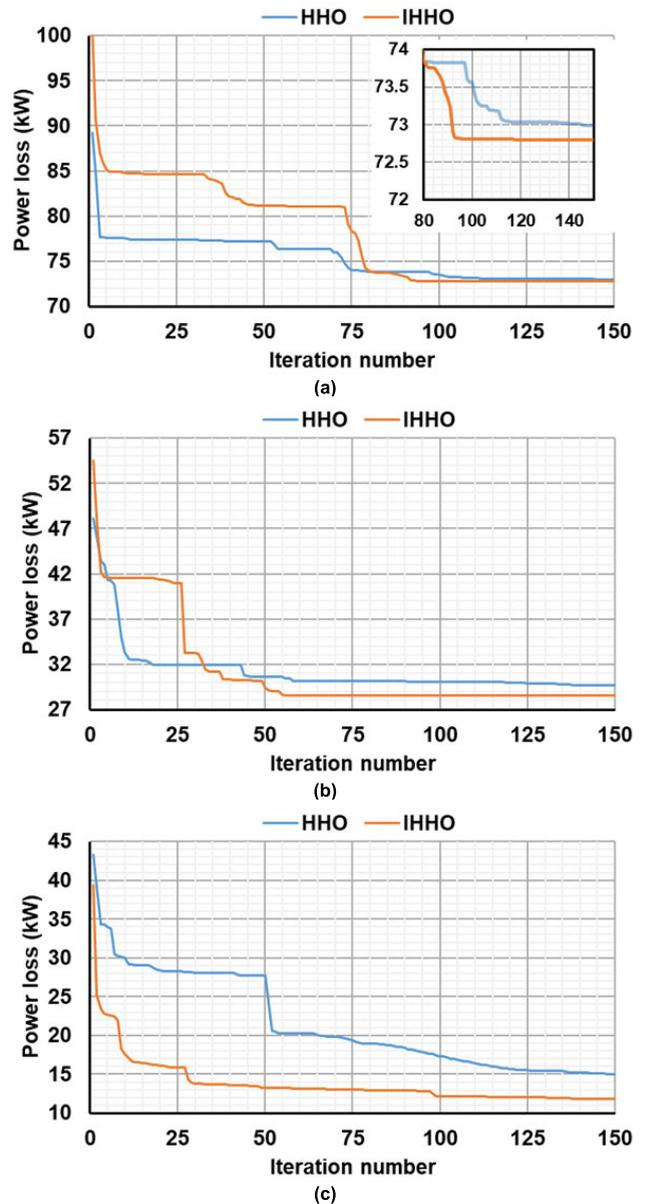
**FIGURE 5.** Convergence characteristics of the HHO and IHHO at different operating p.f for IEEE 33-node test system. (a) unity p.f, (b) 0.95 p.f, and (c) optimal p.f.
