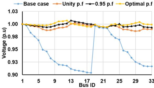
FIGURE 7. Voltage profile of the IEEE 33-node test system at different case studies for the multi-objective optimization problem.
