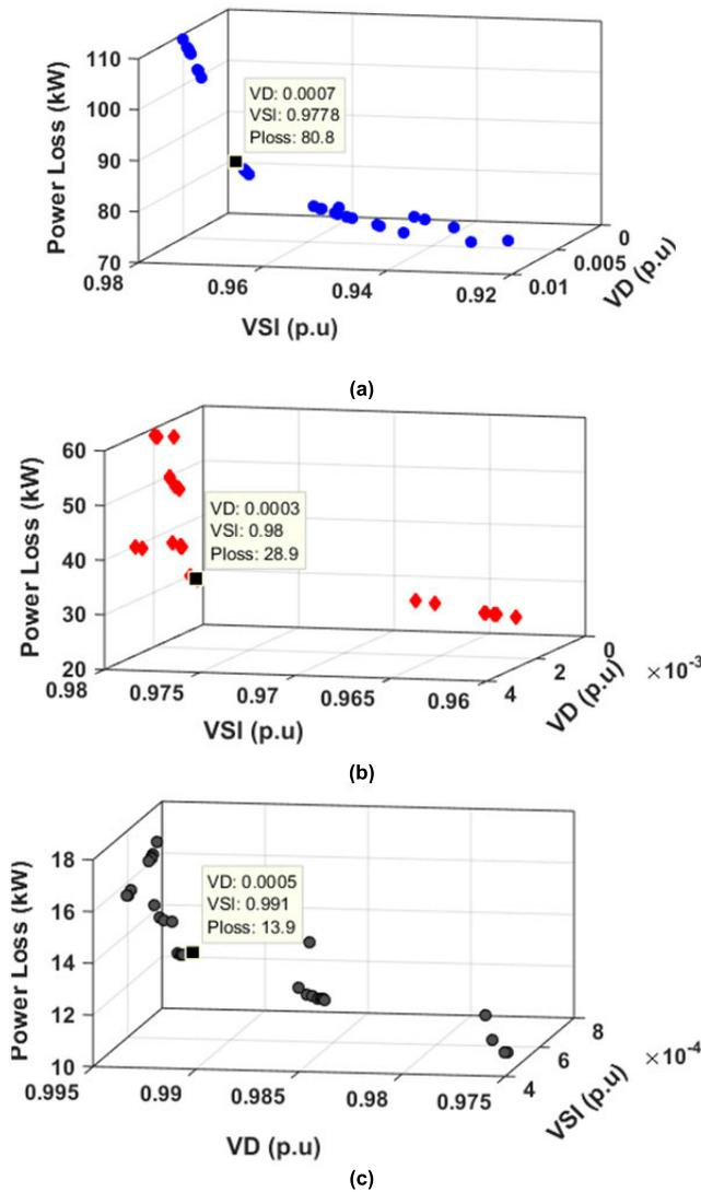
FIGURE 12. Nondominated Pareto optimal solutions obtained by MOIHHO for IEEE 69-bus considering DG operating at: (a) unity p.f, (b) 0.95 p.f, and (c) Optimal p.f.
