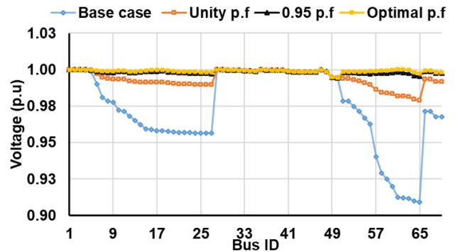
FIGURE 10. Voltage profile of the IEEE 69-node test system at different case studies for the single-objective optimization problem.
