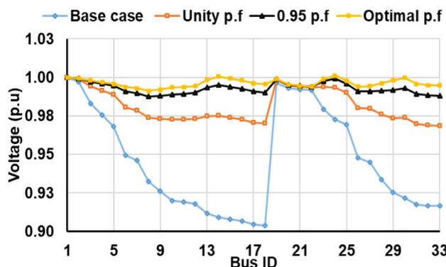
**FIGURE 4. Voltage profile of the IEEE 33-node test system at different case studies for the single-objective optimization problem.**
