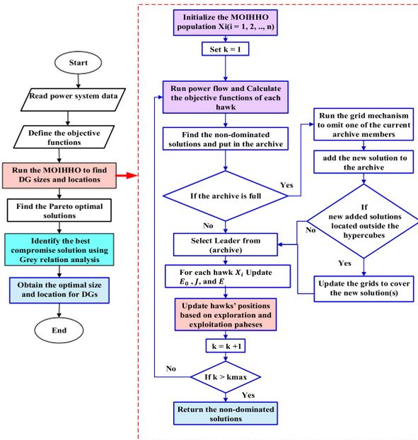
FIGURE 2. MOIHHO for optimal allocation of DG in a distribution network.
