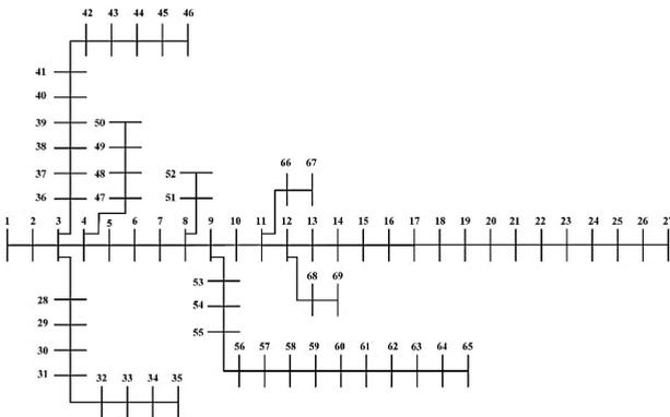
FIGURE 9. Single line diagram of the IEEE 69-node test system.
