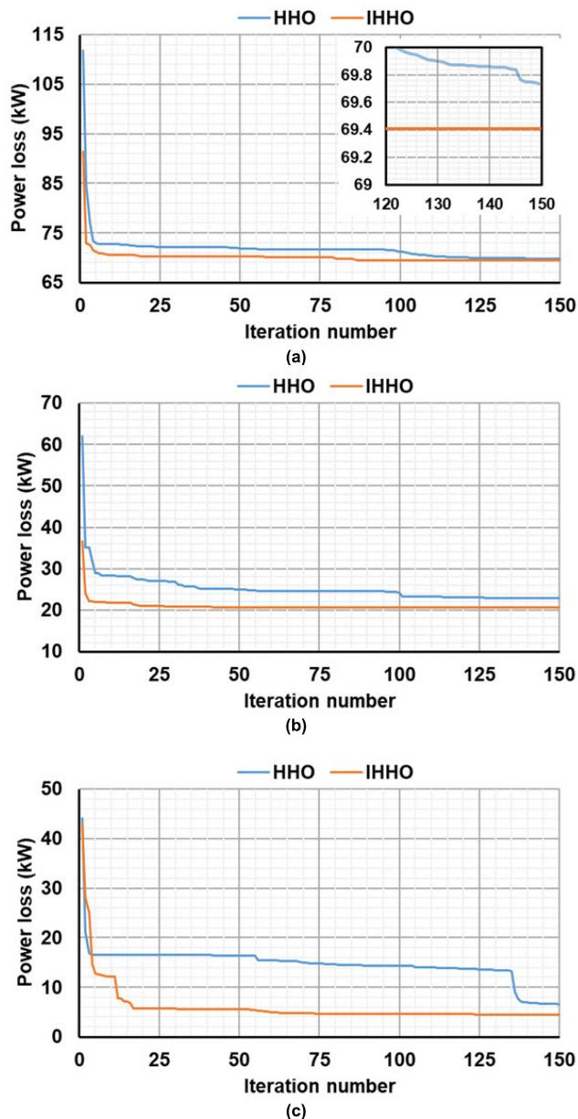
**FIGURE 11.** Convergence characteristics of the HHO and IHHO at different operating p.f for IEEE 69-node test system. (a) unity p.f, (b) 0.95 p.f, and (c) optimal p.f.
