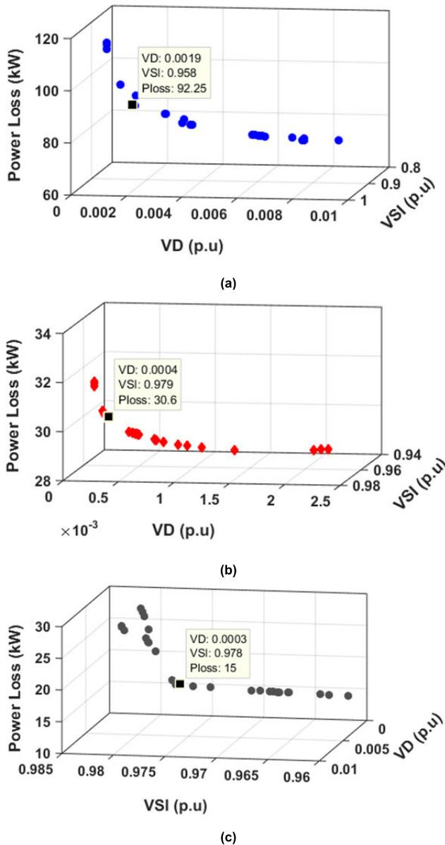
**FIGURE 6.** Nondominated Pareto optimal solutions obtained by MOIHHO for IEEE 33-bus considering DG operating at: (a) unity p.f, (b) 0.95 p.f, and (c) Optimal p.f.
