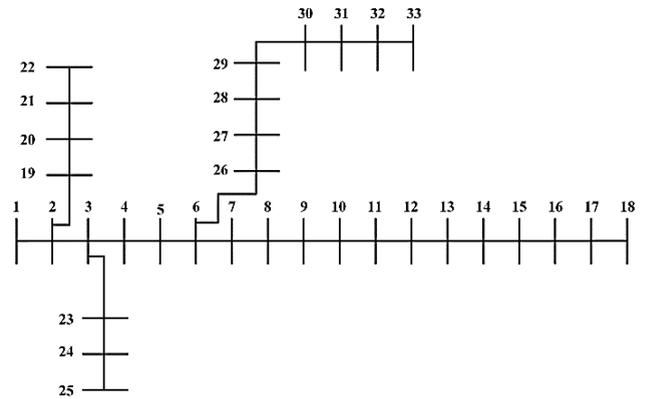
FIGURE 3. Single line diagram of the IEEE 33-node test system.
