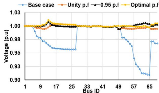
FIGURE 13. Voltage profile of the IEEE 69-node test system at different case studies for the multi-objective optimization problem.
