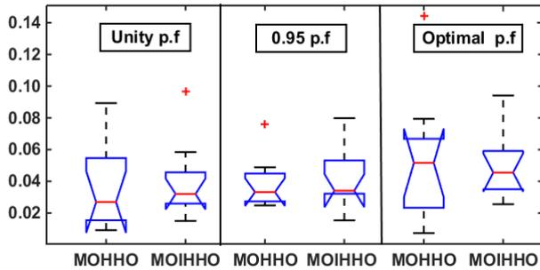
FIGURE 8. Box plot for SP metric of the MOHHO and MOIHHO at different operating p.f. in case of the IEEE 33-node system.
