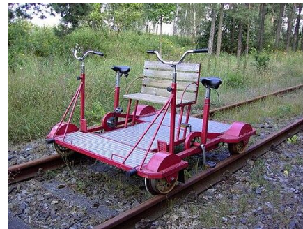
شکل ۱- Two-person rail-cycle draisine with four wheels
