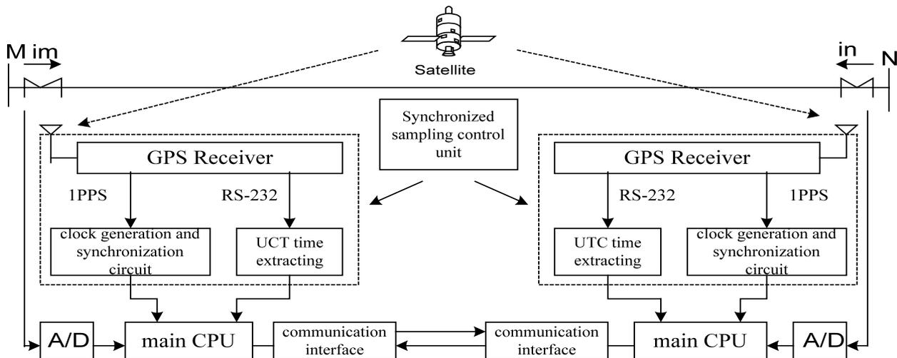
Fig. 1. Block diagram of GPS based current differential protection.
