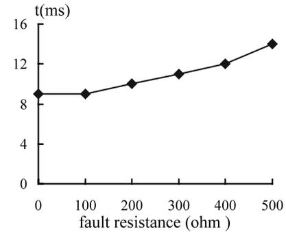
Fig. 6. Tripping time comparison for phase A to earth faults with different fault resistances.
