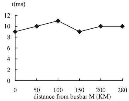
Fig. 5. Tripping time comparison for B–C phase faults ( $R_f = 10 \Omega$ ) at different positions.
