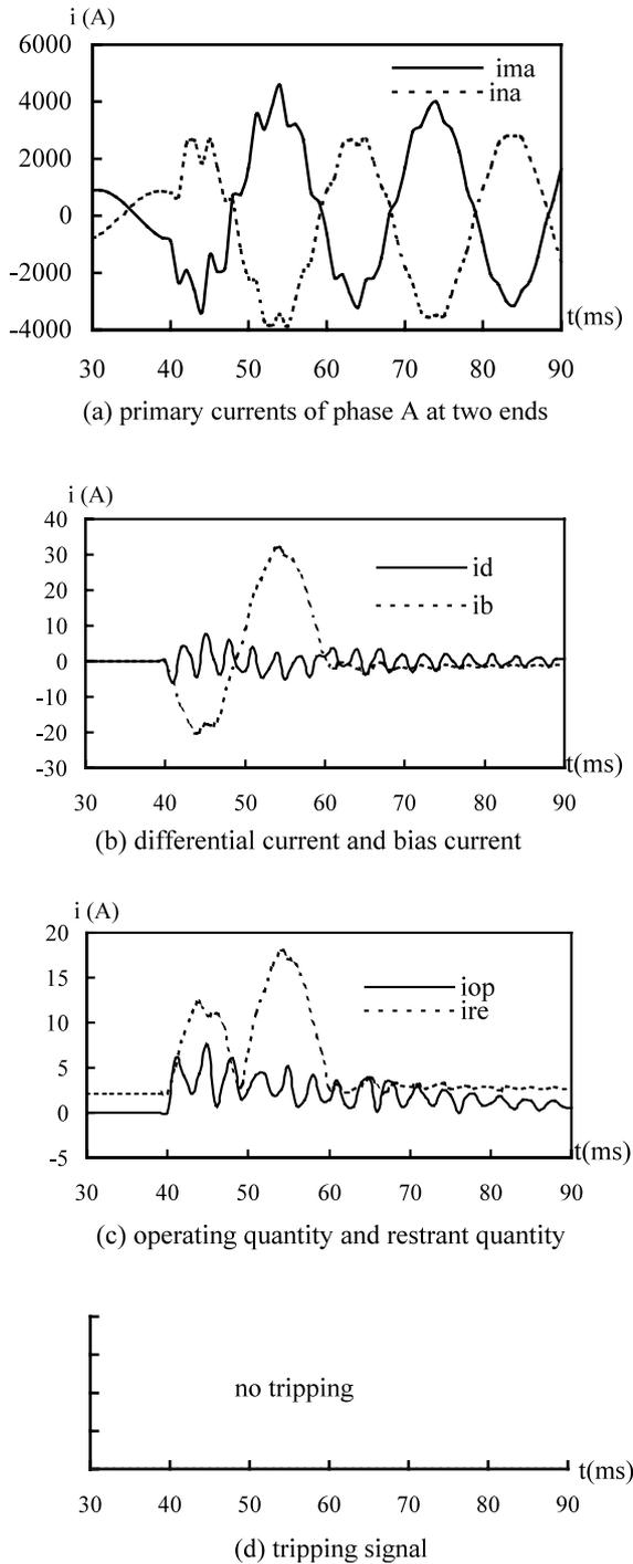
Fig. 7. Response for phase A to earth fault at busbar M.
