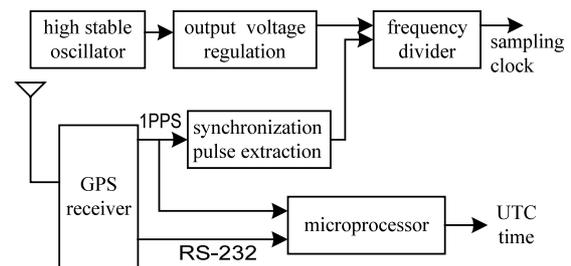
Fig. 2. Synchronized sampling control unit.
