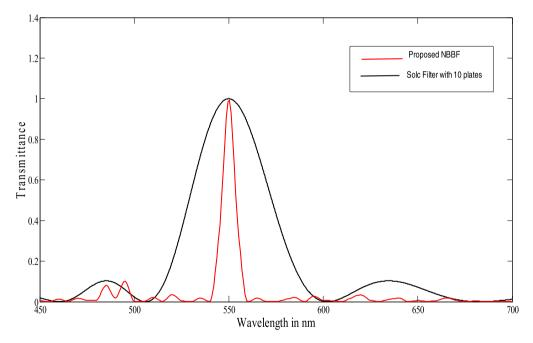
**Figure 7.** Comparison of transmission curve for the proposed filter with the exit polariser rotated at 235° angle (red curve) and that for the filter of [6] with crossed polariser (black curve).
