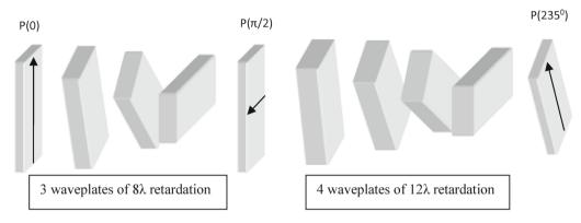
Figure 2. Schematic diagram for the internal arrangement of the proposed narrow band-pass birefringent filter.
