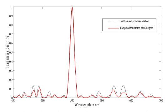
**Figure 6.** Comparison of transmission curve for the proposed filter with exit polariser rotated at 55° angle (black curve) and that for polariser without rotation (red curve).
