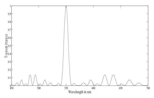
Figure 3. Transmission characteristics for the proposed NBBF with the exit and entrance polarisers in parallel position.
