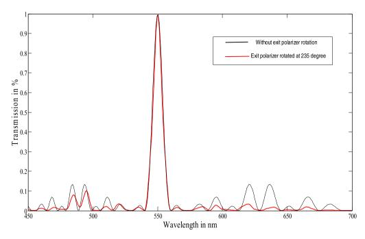
**Figure 5.** Comparison of transmission curve for the proposed filter with exit polariser rotated at 235° angle (black curve) and that for the polariser without rotation (red curve).
