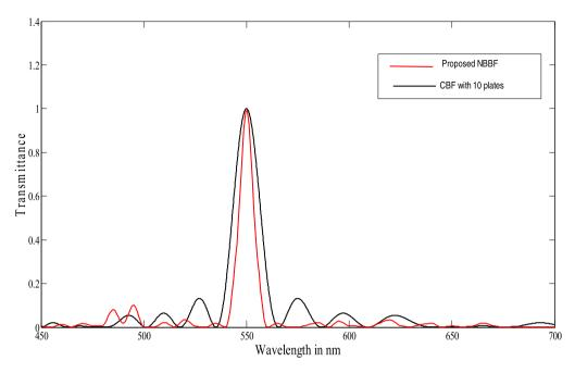
**Figure 8.** Comparison of transmission curve for the proposed filter with the exit polariser rotated at 235° angle (red curve) and that for the CBF (black curve).
