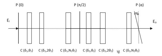
Figure 1. Block diagram of the proposed narrow band-pass birefringent filter.
