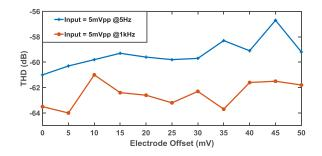
Fig. 17. Measured THD versus electrode offset for a  $5\text{-mV}_{pp}$  input at 5 Hz and 1 kHz separately.
