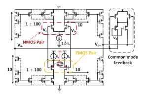
Fig. 5. Schematic of the proposed VLT OTA with a complementary input stage.
