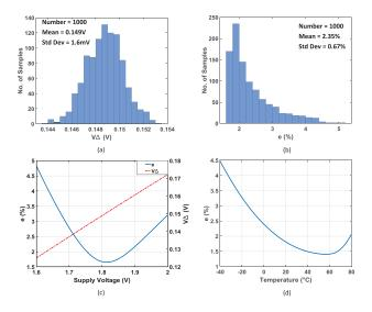
Fig. 7. Simulation results of (a)  $V_{\Delta}$  versus process variations, (b) *e* versus process variations, (c) *e* versus supply voltage, and (d) *e* versus temperature.
