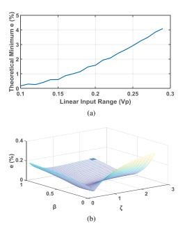
Fig. 6. Plot of (a) linear input voltage versus the achievable minimum nonlinearity *e*. (b) *e* versus  $\beta$  and  $\zeta$ .
