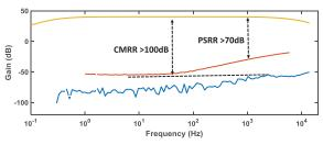
Fig. 18. Measured CMRR and PSRR.
