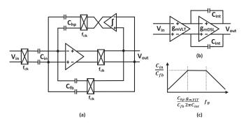
Fig. 1. (a) Schematic of the chopper-stabilized amplifier, consisting of a lownoise OTA and a DSL. (b) Active Gm-C integrator used in DSL. (c) Transfer function of the chopper amplifier using the active Gm-C integrator.
