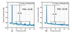
Fig. 16. (a) Measured harmonic distortion of the amplifier for a  $5\text{-mV}_{pp}$  input at 5 Hz. (b) Measured harmonic distortion of the amplifier for a  $5\text{-mV}_{pp}$  input at 1 kHz.
