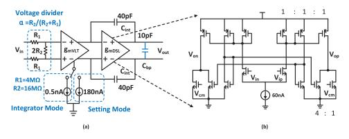
Fig. 11. (a) Architecture of the dc servo loop based on the Gm-C structure. A voltage divider is used as the input stage of the integrator to improve the linearity. (b) Schematic of the OTA  $g_{mDSL}$  used in DSL. A class-AB structure is used.
