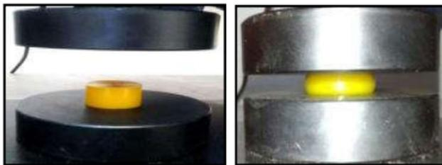
Fig. 2 Compression test of the elastomer
