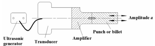
Fig. 1. Schematic of the ultrasonic assisted metal forming processing.
