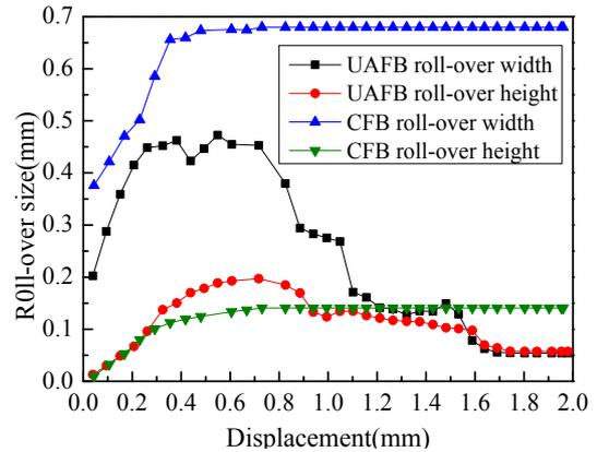
Fig. 11. The roll-over size variation during the whole fine blanking process.
