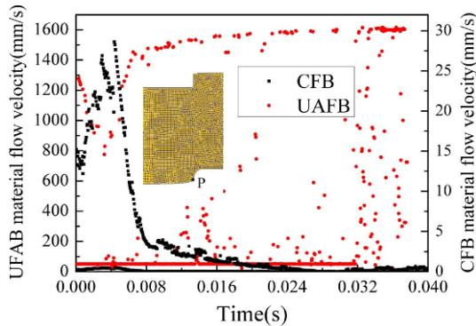
Fig. 8. The metal flow velocity variation at point P for the two forming processes.
