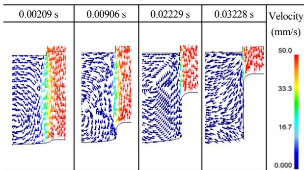
punch in every cycle in the UAFB process. When the billet separated from the punch, the material in shearing zone flowed up, when the billet contacted with the punch, the metal in shearing zone flowed down. This means that ultrasonic vibration changed the material flow direction in the UAFB process.
