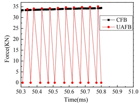
Fig. 6. Fluctuation of punch force due to the vibration.
