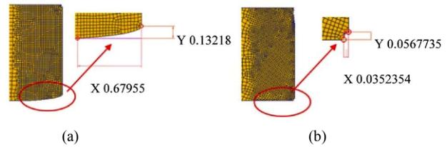
Fig. 10. The size of roll-over: (a) In the CFB process; (b) in the UAFB process.
