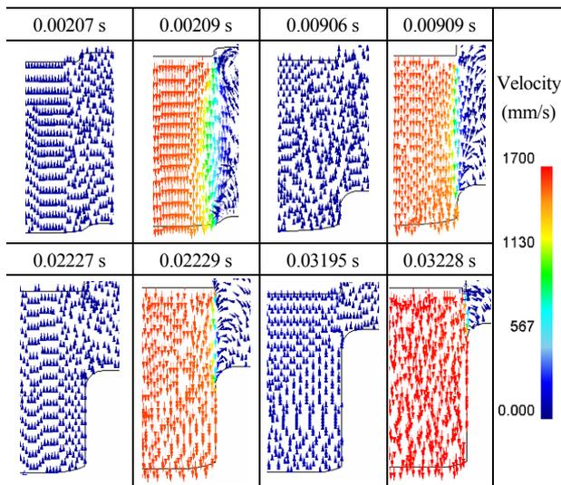
Table 3. The metal flow velocity distribution in shearing zone during CFB process.
