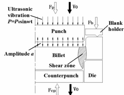
Fig. 2. Schematic of the ultrasonic vibration assisted fine blanking process.
