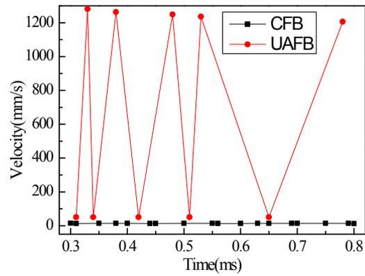
Fig. 9. The metal flow velocity fluctuation diagram.
