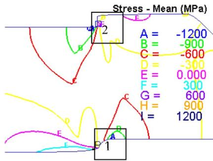
Fig. 12. The material mean stress distributions in the CFB process.
