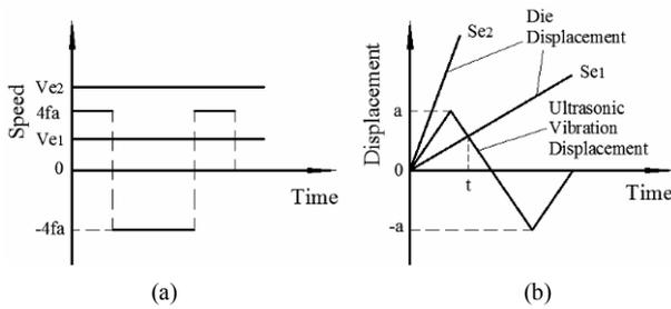
Fig. 7. The UAFB speed and displacement diagram: (a) Variations of fine blanking and vibration speed; (b) variations of punch and die vibration displacement.
