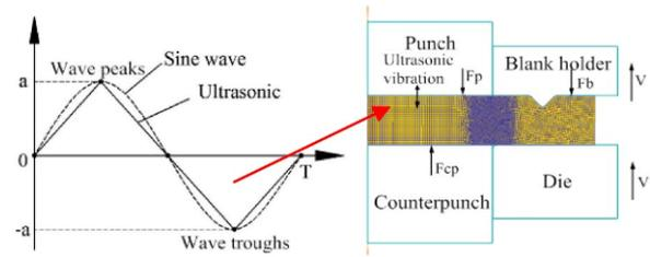
Fig. 4. The FE model of the UAFB process.
