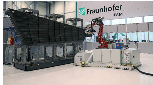
Fig. 14 The mobile robot is processing the tail-fin of an Airbus 320 aircraft. (Courtesy of Fraunhofer IFAM)
