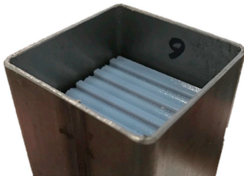
Fig. 4. Region of free space located at the top of each filled TW tube, highlighting the difference in the lattice and tube length.
