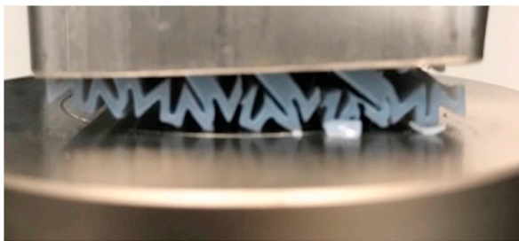
Fig. 16. Lattice protruding from tube.
