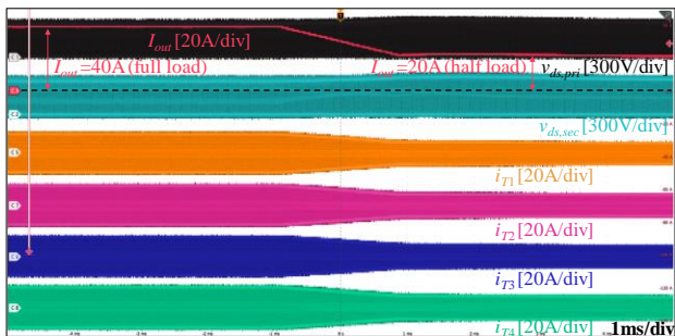
Fig. 12 Load changing test from full load (12 kW) to half load (6 kW).
