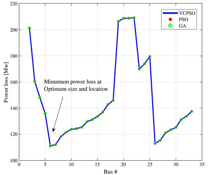
Fig. 8. Active power loss with one optimal DG at different placement
