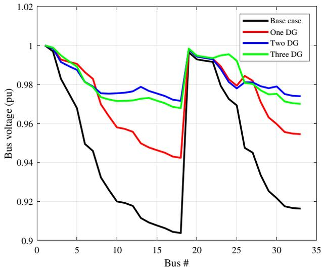
Fig. 10. Variation of bus voltages with different scenarios
