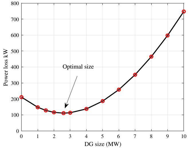
Fig. 12. Power loss characteristic with DG size variations
