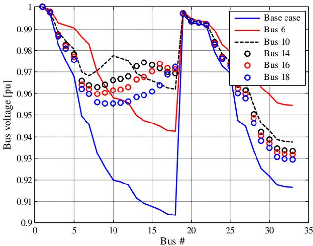
Fig. 11. Variation of bus voltages without and with optimal one DG integration
