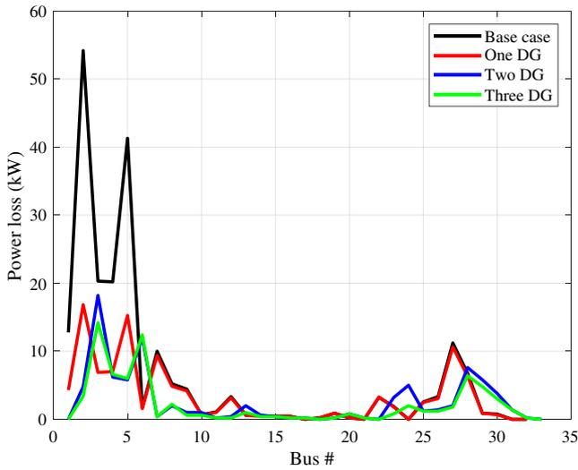
Fig. 9. Total active power loss variations with different scenarios
