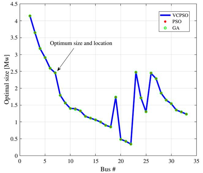
Fig. 7. Different optimal DG sizes at different placements
