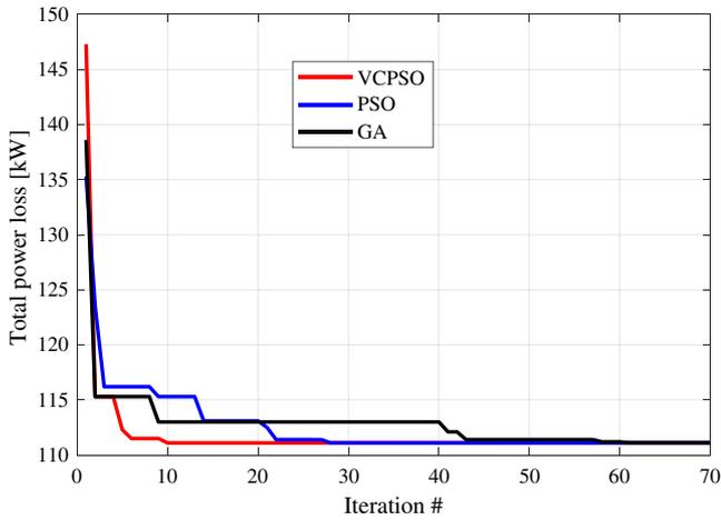
Fig. 6. Convergence characteristics of presented algorithms
