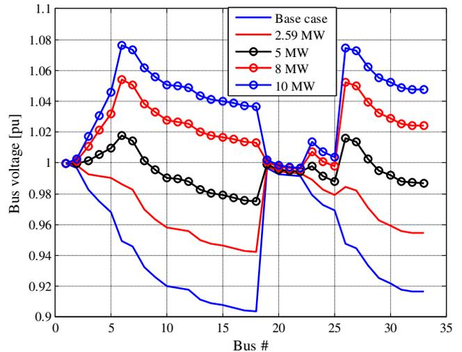
Fig. 13. Variation of bus voltages with non-optimal DG size
