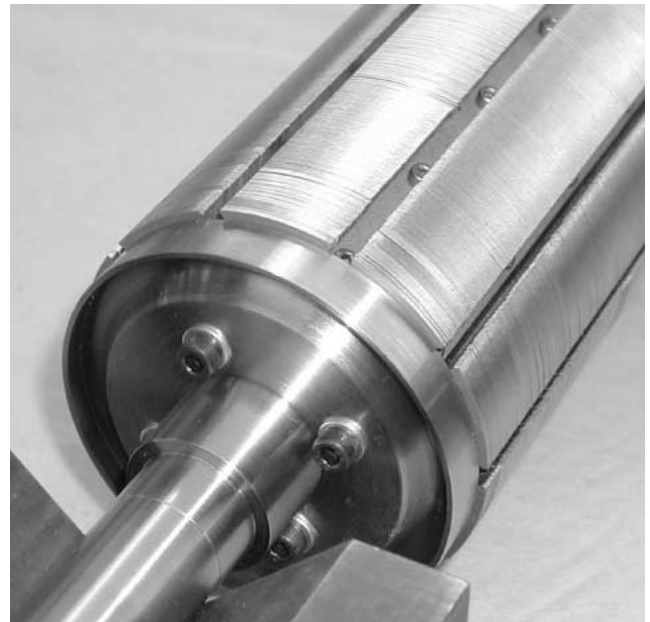
Fig. 6 Rotor of 12-10 single-tooth SRM, showing individual rotor segments
