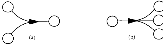
Fig. 2. (a) A B-arc. (b) An F-arc.
