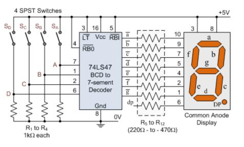
The connection between the 74LS47 decoder/driver and the common anode display, requires seven resistors (eight if the decimal point is included) to limit current flow. For each LED segment of the display to light properly, the flow of current through each segment needs to be carefully controlled.
