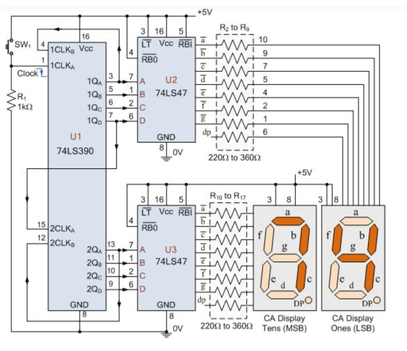
The circuit shows a simple 00 to 99 digital counter using a 74LS390 BCD Counter and two 74LS47 7-segment display drivers. To count above 99, we would need to cascade more counter circuits together.
