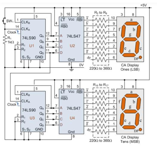
So how does this 2-digit 7-segment display counter work. The first half of the digital counter circuit works the same as before except that the activation of the pushbutton SW<sub>1</sub> increments the "one's" (also called "units") LED display.
