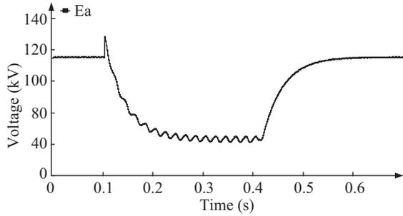
Fig. 1. Characteristics of voltage sags caused by lightning.
