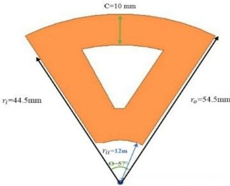
Fig 6. Stator coil
