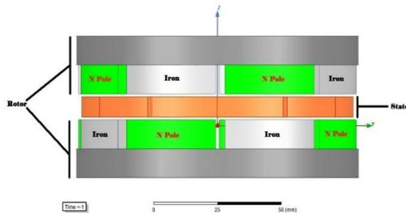
Fig 1. Structure of the proposed model
