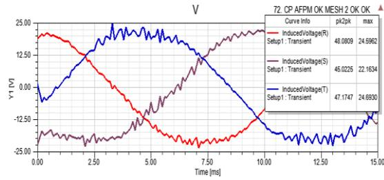
**Fig 14.** Induced voltage of a toothed consequent pole sector generator
