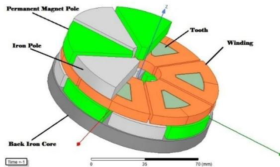
Fig 2. Side view of the proposed model
