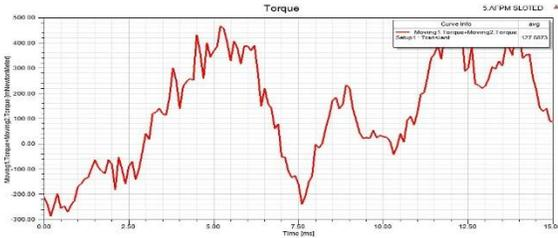
**Fig 17.** Cogging torque in toothed sector generator
