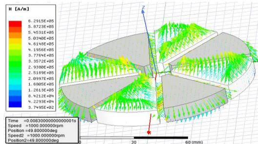
**Fig 10.** Flux movement towards the teeth
