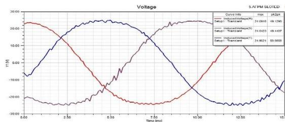
**Fig 13.** Induced voltage of toothed sector generator
