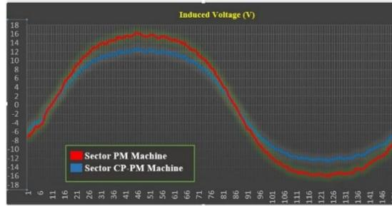
**Fig 9.** Induced voltage of sector generator and the sector consequent pole
