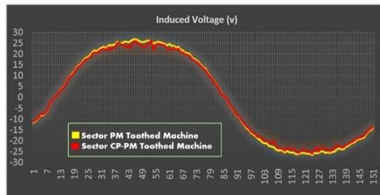
**Fig 15.** Induced voltage of toothed sector generator and toothed consequent pole sector generator
