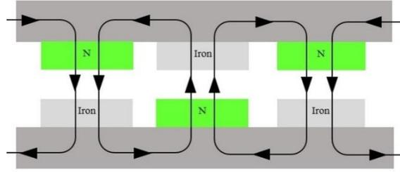
**Fig 3.** Magnetic flux path
