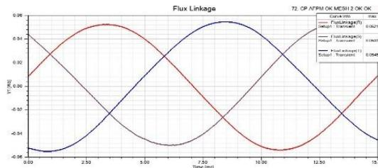
**Fig 16.** Linkage flux of CP-PM generator
