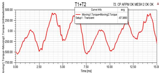
**Fig 18.** Cogging torque in toothed consequent pole sector generator
