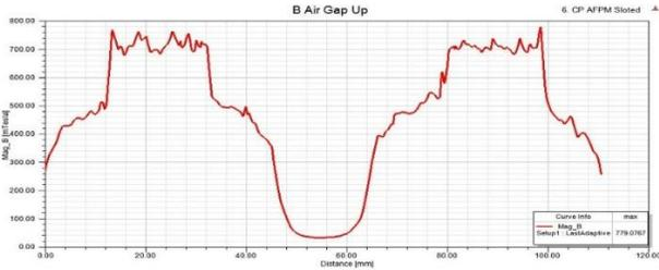
**Fig 18.** Flux density in the air gap of the in toothed consequent pole sector generator
