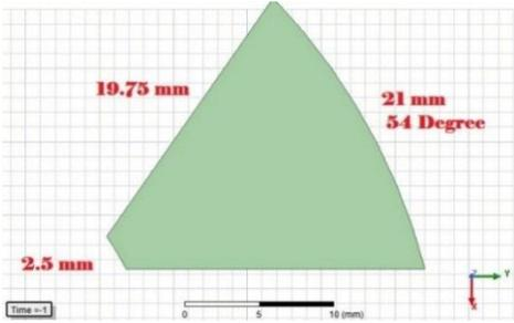
Fig 7. Stator tooth
