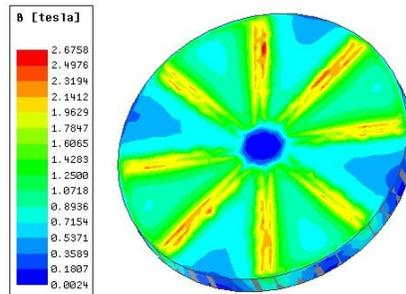
**Fig 12.** Flux density in the back plate the CP-PM generator poles
