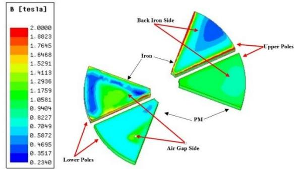
**Fig 11.** Magnetic flux density in CP-PM generator poles
