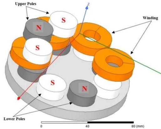
**Fig 8.** Machine structure with circular poles and windings
