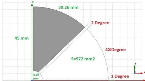
**Fig 5.** The dimensions of the sector poles
