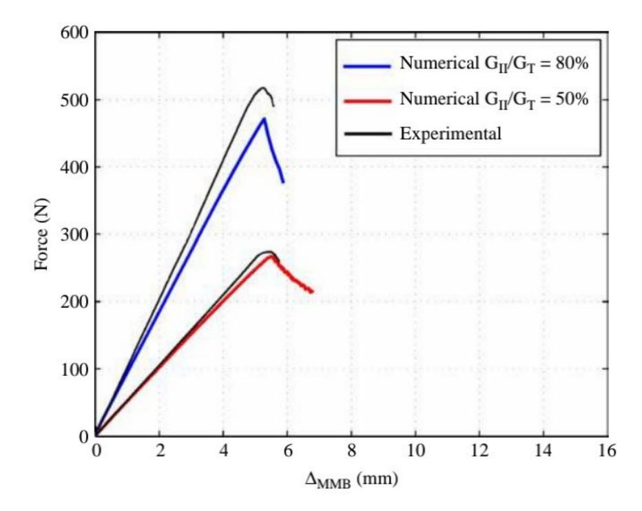
Figure 9. MMB test, numerical-experimental comparison
