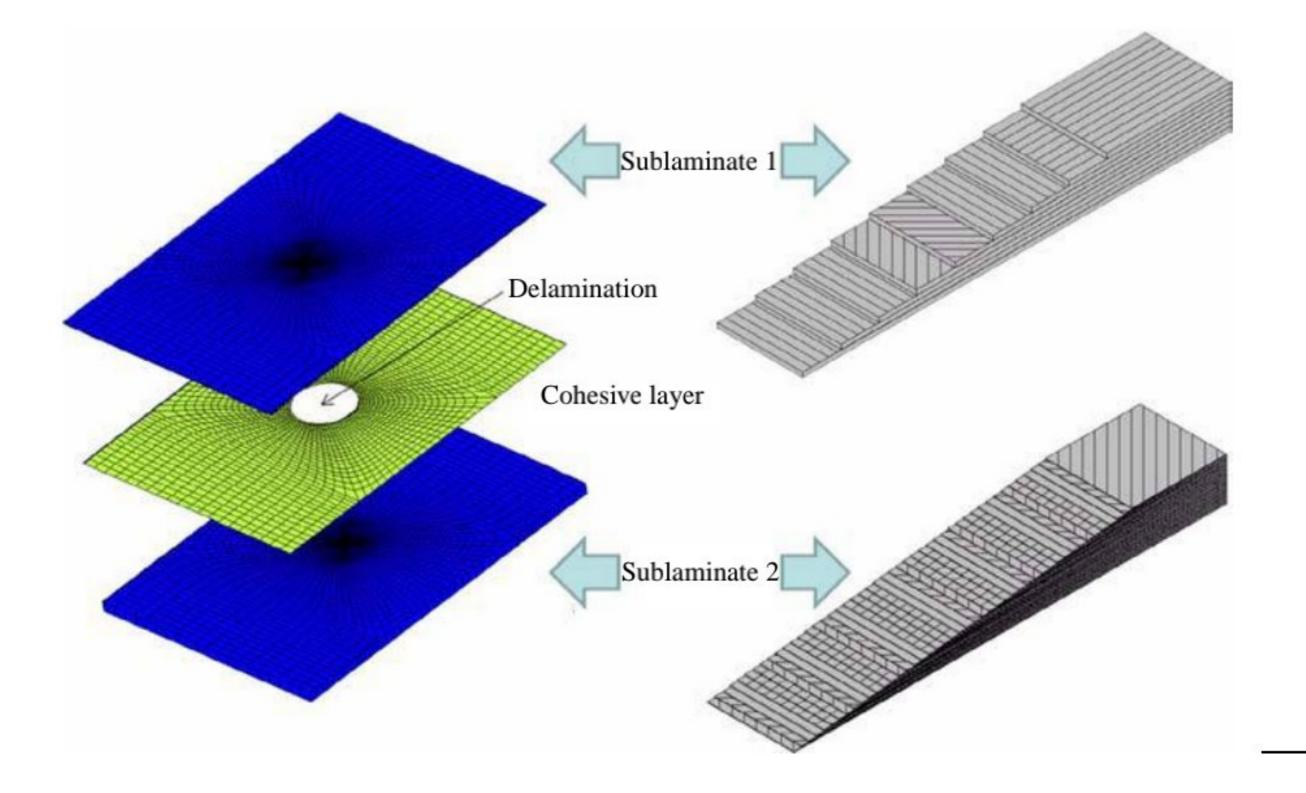
Figure 11. FE model of a skirt's specimen
