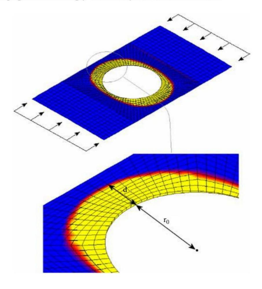
Figure 14. Damage evolution band plot (cohesive layer)
