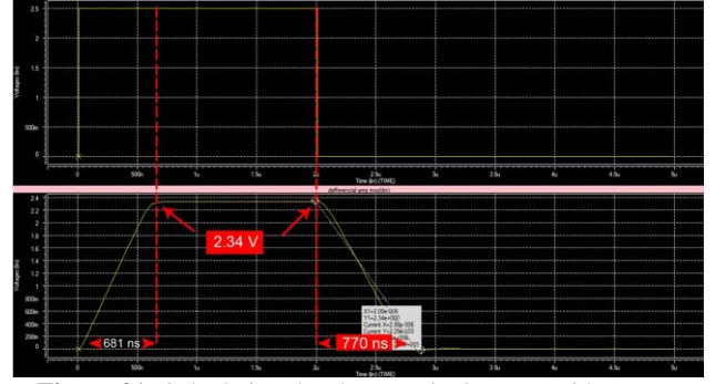
Figure 21. Calculating the slew rate in Op-amp with current buffer and miller capacitor
