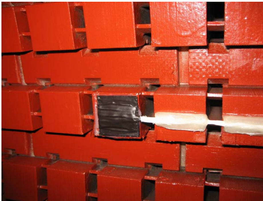
Figure 1. New style flat flux probe mounted on a tooth
