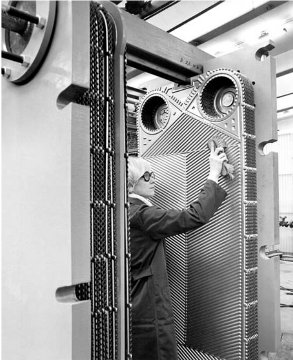
FIGURE 11.8 Cleaning the plates. (Courtesy of Alfa-Laval Thermal AB.)
