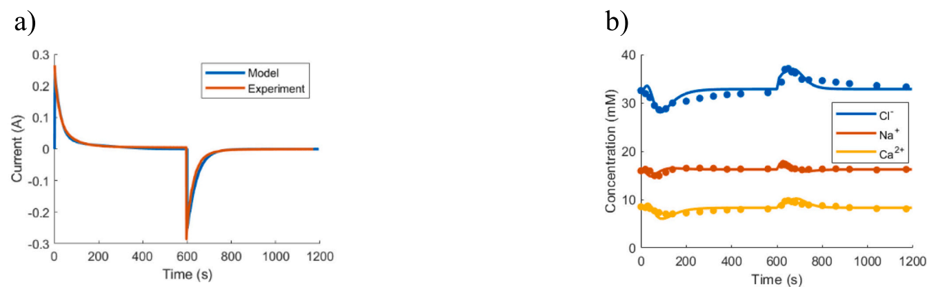
Fig. 5. The operation of an FCDI device. The experiment data are from Ref. [26] and the model lines are new. (a) This is the measured current, based on CV charging and discharging. (c) The measured effluent concentration from the device for each of the ionic species. The dots correspond to the experimental data and the lines are from the model.
