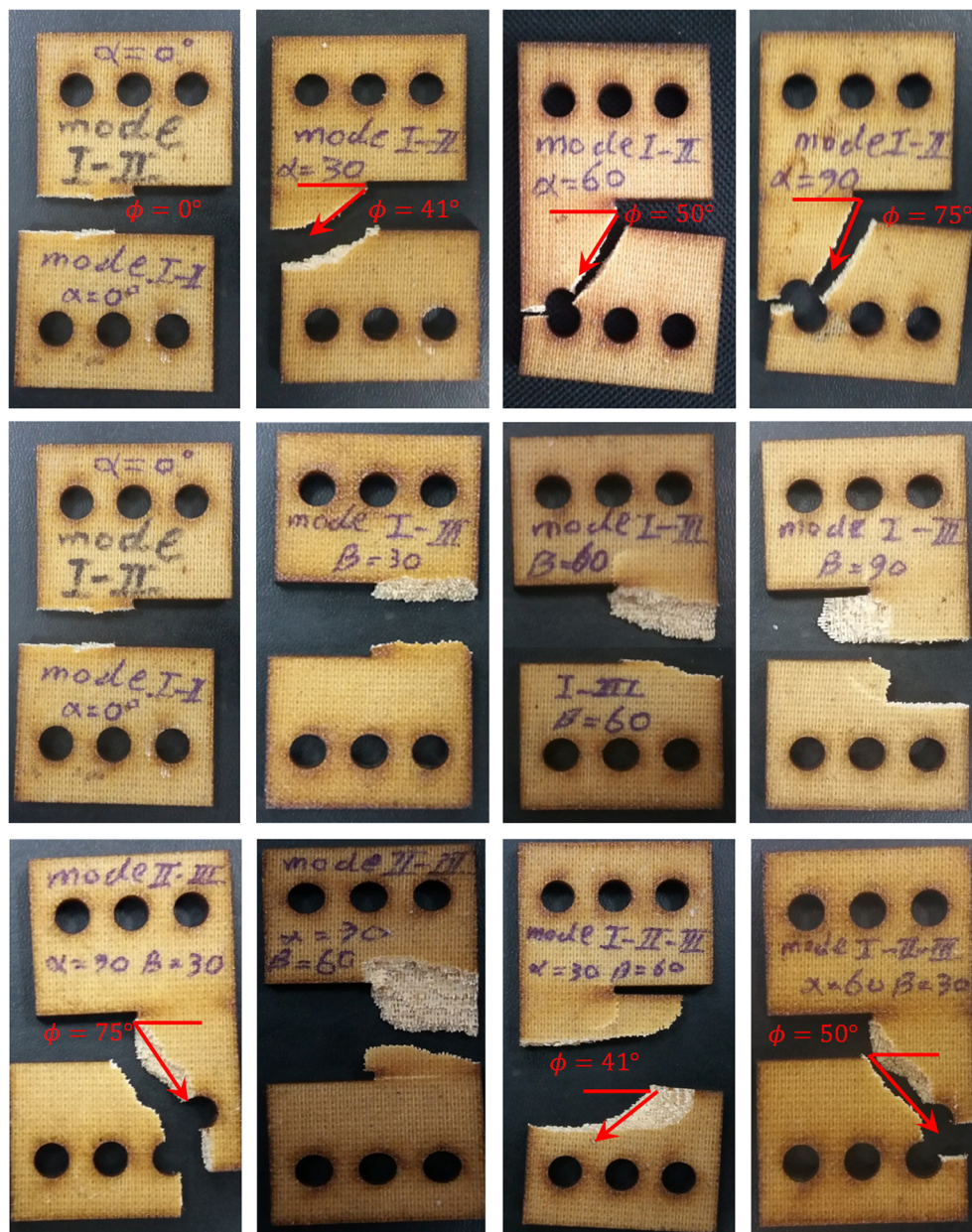
Fig. 13. Typical fracture profile of the CTS specimens made of cotton/epoxy system under different loading angles.
