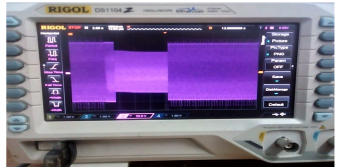
Fig. 15. Hardware result in SAG creation and clearing with UPQC.
