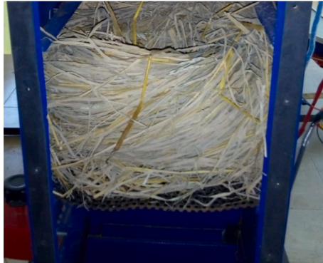
Fig. 3. Picture of the paddy grass packing material in the humidifier.
