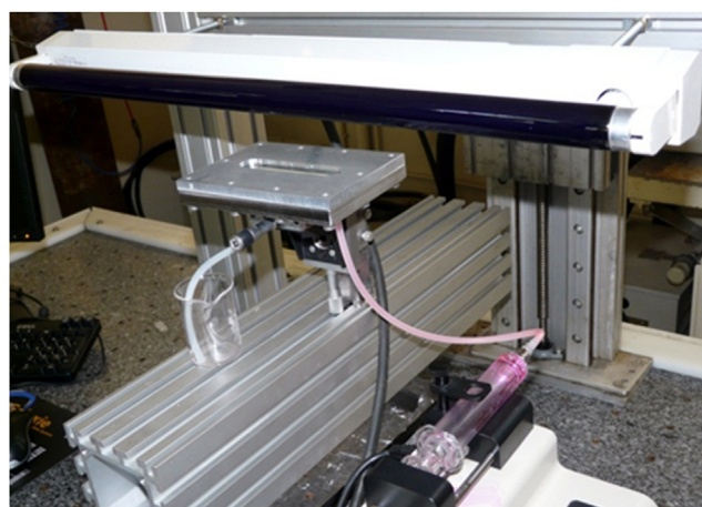
Fig. 2 – Experimental setup equipped with feed control consisting of a syringe pump system.
