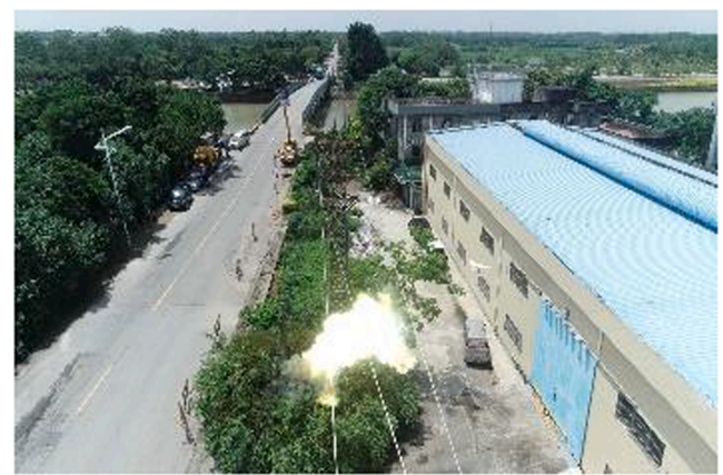
Fig. 22. The artificial short-circuit test.
