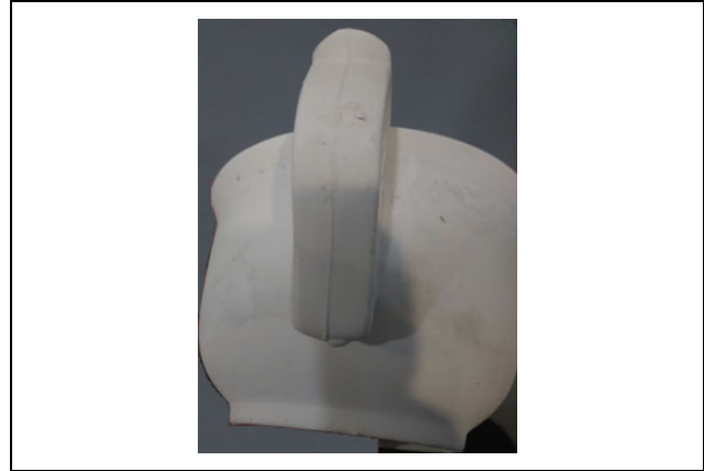
Figure 1. Polishing/fettling: removal of excess ceramic materials.
