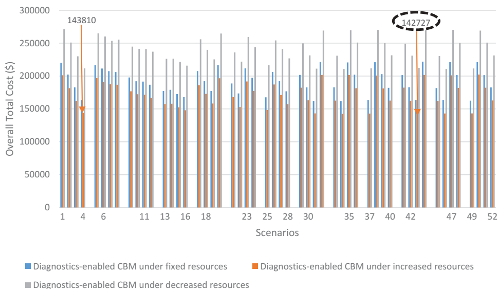
Figure 10. Effect of MCR under diagnostics-enabled CBM policy with fixed resources, increased resources, and decreased resources on overall total cost.
