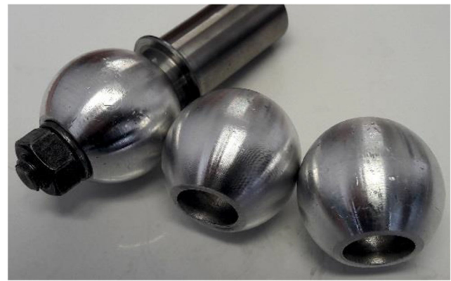
Fig. 26 Examples of finished products obtained from hollow balls with the use of a chuck (shown in the photograph) and a CNC lathe
