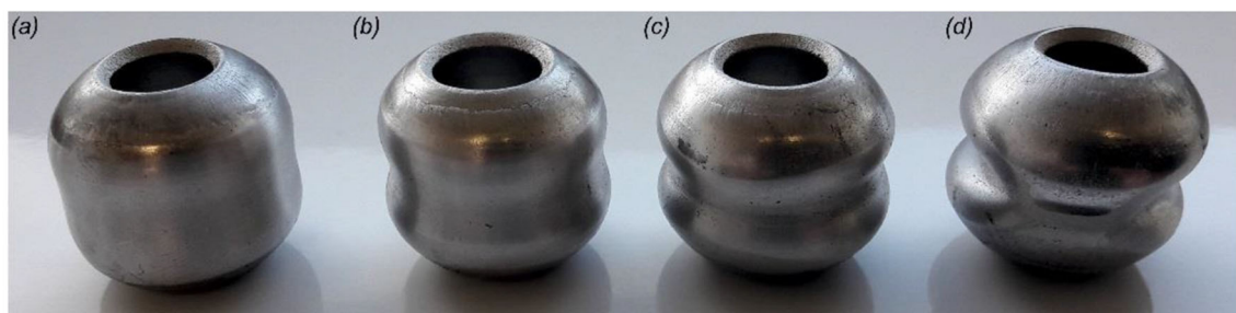
Fig. 2 Examples of hollow balls formed from a tube with a thickness g_0 of 2 mm, an outside diameter d_0 of 26 mm and heights h_0 of (a) 31.0 mm, (b) 31.7 mm, (c) 34.4 mm and (d) 37.2 mm, respectively (the balls shown in this figure were obtained in preliminary studies)
