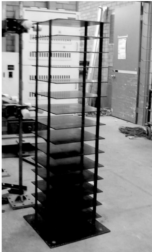
Figure 6. Completed structural model
