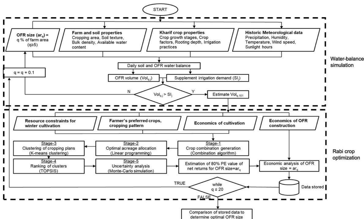
Fig. 2. Step-by-step exposition of the proposed simulation-optimization scheme.
