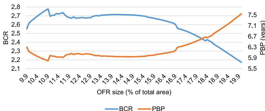
Fig. 5. Benefit Cost ratio (BCR) and Payback period (PBP) of different sizes of On-farm reservoir (OFR).
