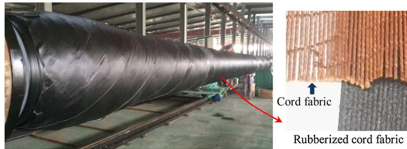
Fig. 3. Rubberized cord fabric wound on mandrel.
