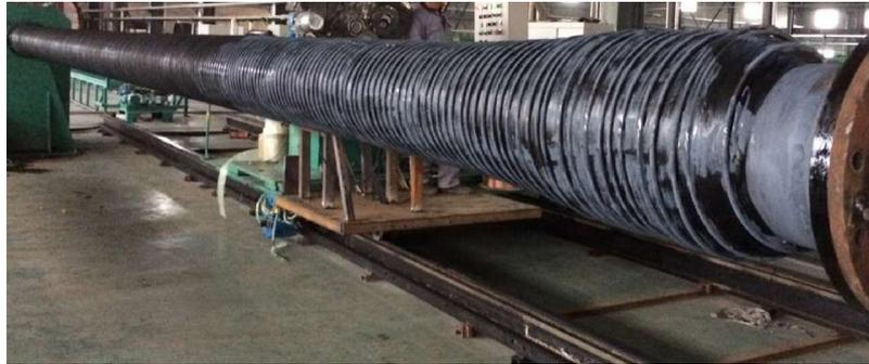
Fig. 4. Steel stiffener wound on the hose.
