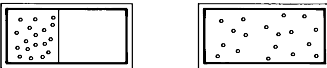
Figure 2-2. The initial and final states of the expansion of a gas into a vacuum.
