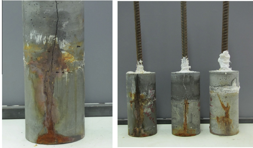
Fig. 6. Typical corrosion specimens after the accelerated corrosion test.
