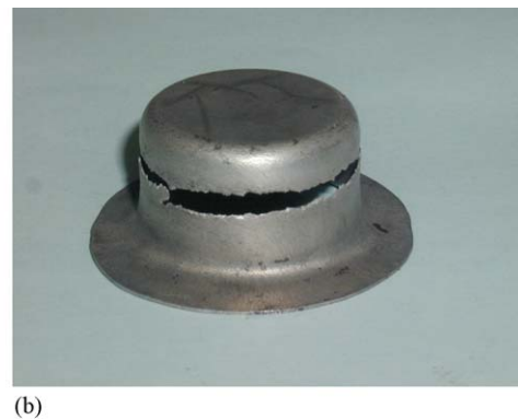
Fig. 12. Comparison between FEM simulation and experimental results (material properties of blank at 300 °C in FEM): (a) FEM simulation ( BHF_{const} = 6.0 kN, DR=2.1, \mu=0.05 ); (b) experiment ( BHF_{const} = 5.88 kN, DR=2.1, 300 °C).
