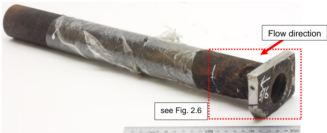
Fig. 2.5: Overview of the cut tube as seen in Fig. 2.2. Tube from 6 th row, tube No. 5 from furnace 4 C (TL 1411C). The flow direction is shown. Cross section samples were obtained from the red dotted area as seen in Fig. 2.6.
