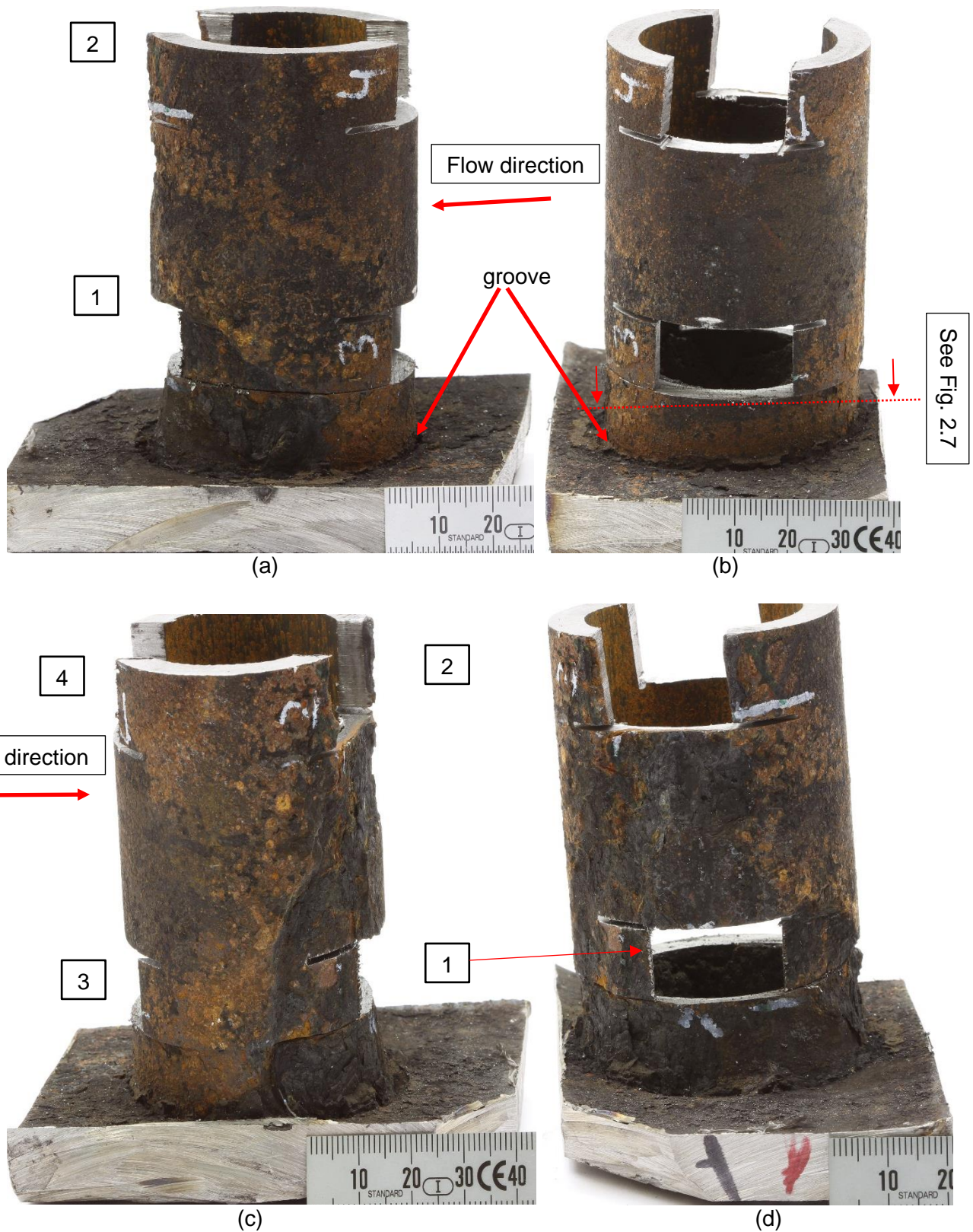
Fig. 2.6: View of samples cut out of tube No. 5 of 6 th row, furnace 4 TLE C (refer to Fig. 2.3). In total 4 samples were cut out for further investigation as seen above. The flow direction is given; hence sample 1 & 2 are at the back of the tube with respect to the flow direction.
