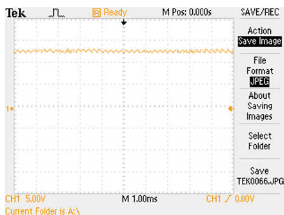
Fig. 3.12 Load voltage with proposed SMC with load 32\ \Omega , \alpha = 6000 , \gamma = 0.0020
