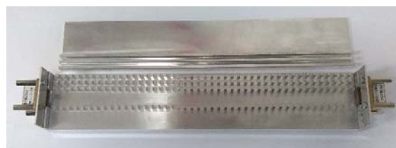
Fig. 9. Gap waveguide leaky wave antenna prototype.
