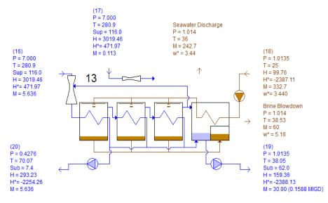
Fig. 5. MED plant, P[bar], T[C], H[kJ/kg], M[t/h]
