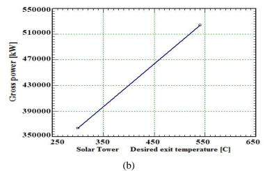
Fig. 6. Gross electric efficiency and gross power
