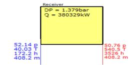
Fig. 2. Solar tower receiver, p[bar], T[C], h[kJ/kg] m[t/h]
