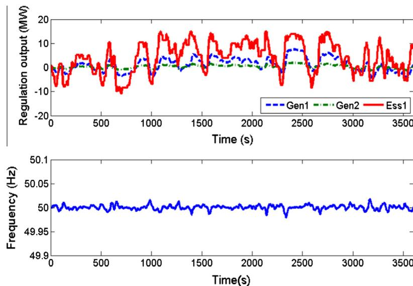
Fig. 5a. Regulation outputs of resources and system frequency response in proposed performance-based regulation market.
