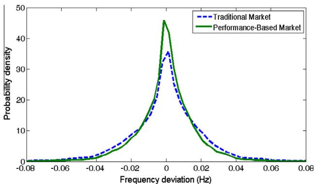
Fig. 8. PDFs of frequency deviations under proposed regulation market design and traditional regulation market neglecting regulation performance.
