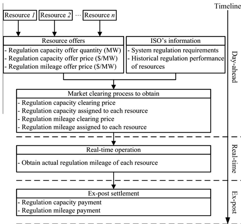
Fig. 1. Scheme of proposed performance-based frequency regulation market.
