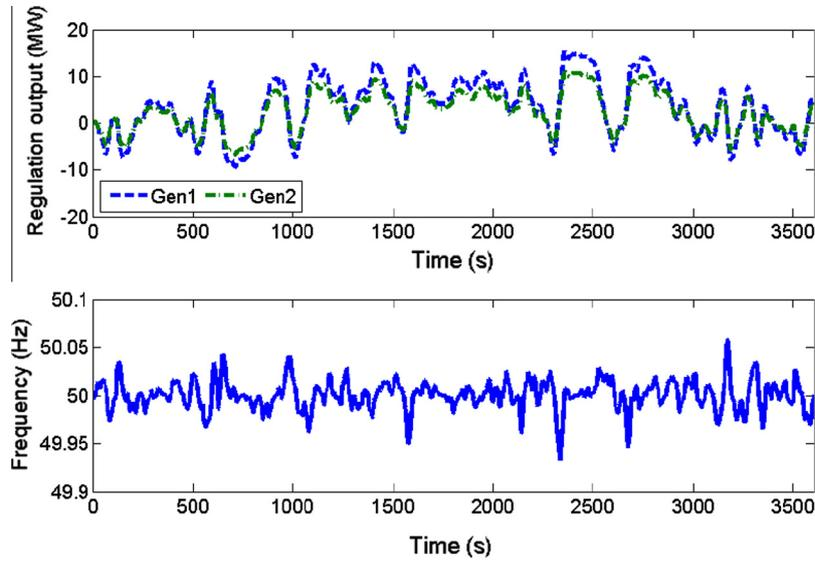
Fig. 5b. Regulation outputs of resources and system frequency response in traditional regulation market neglecting regulation performance.
