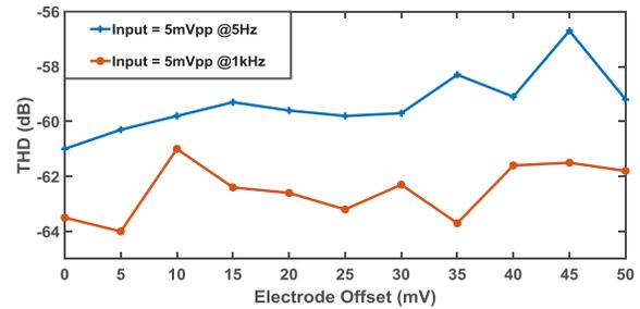
Fig. 17. Measured THD versus electrode offset for a 5-mV<sub>pp</sub> input at 5 Hz and 1 kHz separately.
