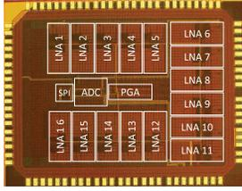
Fig. 13. Microphotography of the proposed chip, which has been fabricated in a TSMC 180-nm CMOS process, occupying a silicon area of 2.6 mm × 2 mm.
