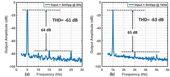
Fig. 16. (a) Measured harmonic distortion of the amplifier for a 5-mV<sub>pp</sub> input at 5 Hz. (b) Measured harmonic distortion of the amplifier for a 5-mV<sub>pp</sub> input at 1 kHz.
