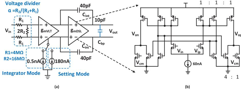
Fig. 11. (a) Architecture of the dc servo loop based on the Gm-C structure. A voltage divider is used as the input stage of the integrator to improve the linearity. (b) Schematic of the OTA  $g_{mDSL}$  used in DSL. A class-AB structure is used.
