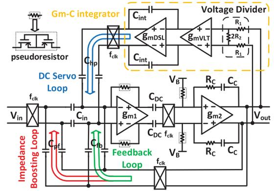
Fig. 9. Schematic of the proposed two-stage chopper-stabilized amplifier.
