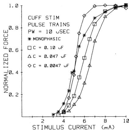
Fig. 10. Special case of the effect of the secondary pulse on the recruitment curves using nerve cuff stimulation. The aberration lies in the fact that the  $0.0047 \mu\text{F}$  curve (diamonds) lies close to the monophasic curve. This is in contrast to the usual result as shown in Fig. 8.
