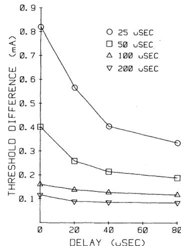
Fig. 2. Nerve model determination of the difference in threshold between 10 and 20  $\mu\text{m}$  fibers ( $I_{10} - I_{20}$ ) for various pulse widths and delay times. All stimuli are rectangular biphasic pulses and the minimum separation between nerve and electrode is 1 mm.
