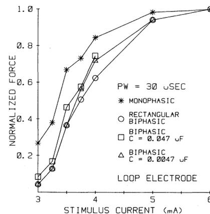
Fig. 6. Comparison of the rectangular and the exponentially decaying secondary pulse with loop electrode stimulation. All curves are normalized to a maximum force of 11.8 N.
