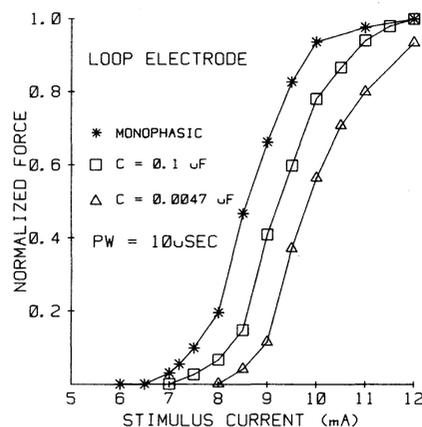
Fig. 5. Effect of inclusion of the secondary anodic pulse with loop electrode stimulation. Capacitor values for the exponentially decaying pulses are indicated. Force normalized to 25 N in all cases.
