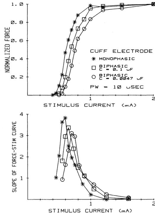
Fig. 8. Effect of inclusion of the secondary pulse with nerve cuff electrode stimulation at narrow (10  $\mu$ s) primary pulse widths. Biphasic curves are shifted to the right of the monophasic curve. Large  $I_s/I_p$  values (small capacitance values) produce greater effects. Monophasic, 0.1  $\mu$ F, and 0.0047  $\mu$ F curves normalized to 17.4, 16.8, and 18.3 N, respectively.
