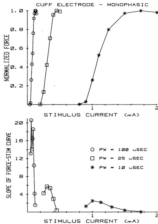
Fig. 7. Effect of pulse width on recruitment curve with nerve cuff electrode stimulation. Monophasic, single pulses used here. Graphs are in same format as Fig. 4. Note the low-stimulus current values relative to loop electrode stimulation. 10, 25, and 100  $\mu$ s curves normalized to 18.3, 27.1, and 33.0 N, respectively.
