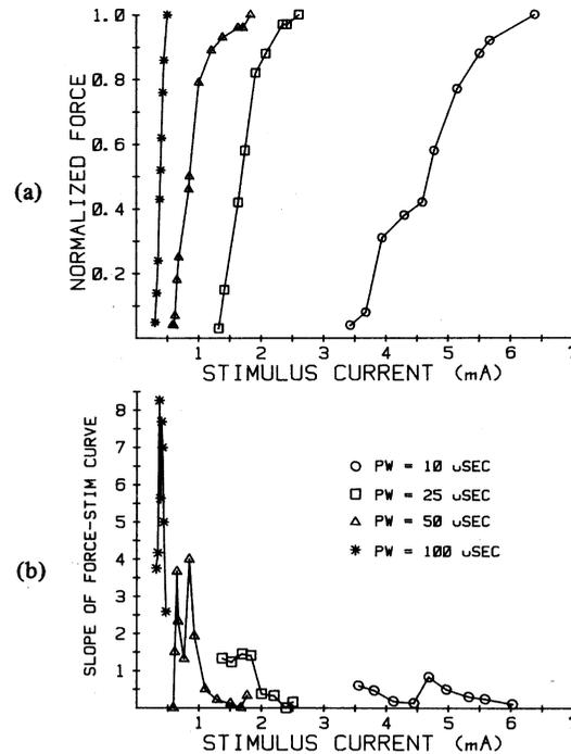
Fig. 4. Effect of pulse width on recruitment curve. Biphasic, zero delay rectangular pulse stimulation through a loop electrode in a saline bath. (a) Actual recruitment curves. Force normalized to 8 N in all cases. (b) Slope of the recruitment curves along their length (in units of normalized force/mA).
